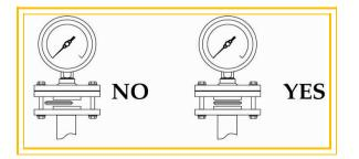
Warning – As gripping hold for the wrench, use the seal side and not the gauge side, in order to prevent leaking of the filling liquid from the seal side In case of threaded connection with exposed
